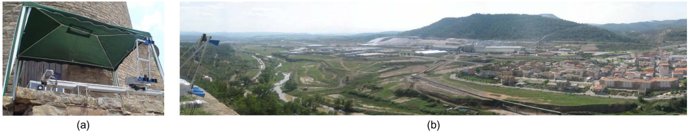
Fig. 1. (a) UPC ground-based SAR sensor and (b) wide-angle view of the test-site from the its location in Sallent.
