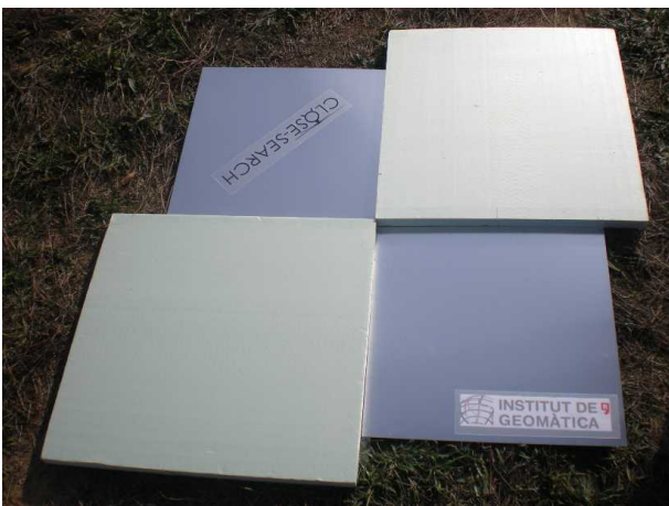
Figure 7: The thermal passive target used during the Test Campaign in CLOSE-SEARCH
