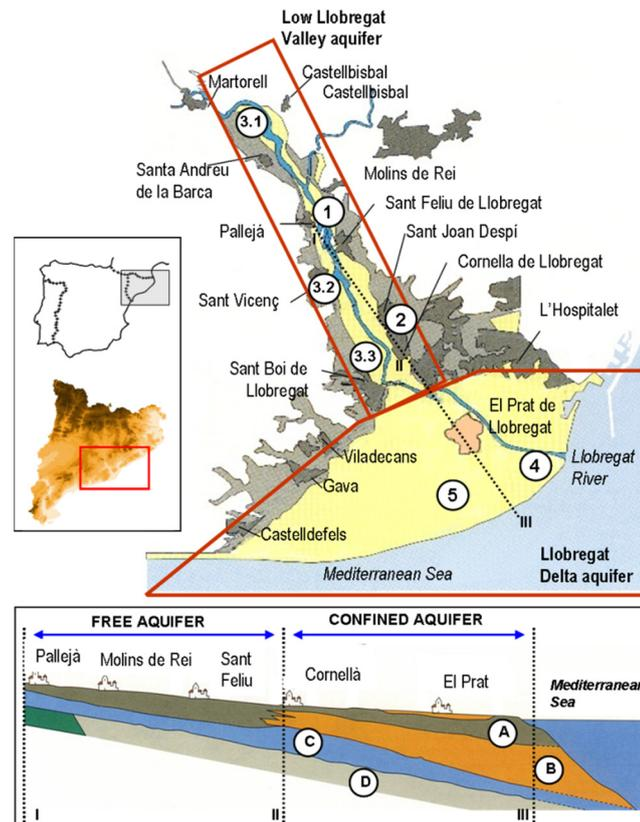
Overview of the Llobregat Delta aquifer. **In the top:** location of the main recharge actions. Sites visited in this field trip: (2) Cornellà, Aquifer Storage and Recovery wells (ASR); (3.2) Sant Vicenç dels Horts infiltration pond and (4) hydraulic barrier. **Bottom:** hydrogeological context. (A) Upper aquifer (sand and gravel); (B) Aquitard (clay and silt); (C) Main aquifer (confined) (sand and gravel); (D) basement previous to quaternary. Source: Modified from Armenter 2008.
