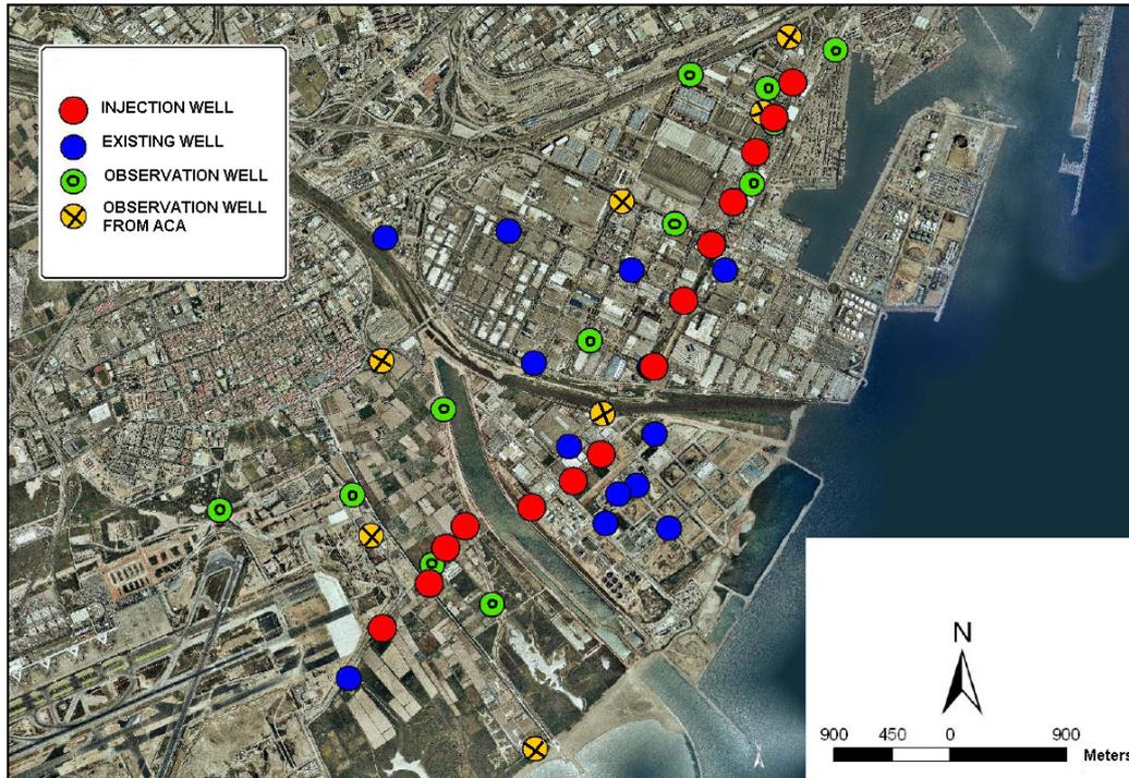
*Monitoring network in the Llobregat hydraulic barrier. There are 14 injection wells, 17 piezometers equipped with temperature and electrical conductivity remote sensors. 7 previously existing piezometers and 12 industrial wells are also located. Source: ACA, 2009.*
