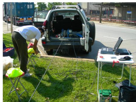
*Well logging surveys in three piezometers of the El Prat de Llobregat Hydraulic barrier.*
