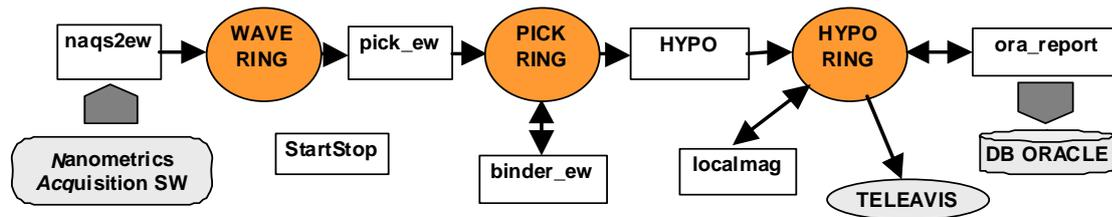
**Figure 3: Simplified diagram of the Automatic Earthworm modules installed at ICC**
