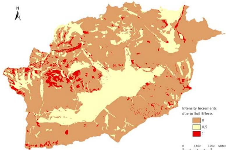
**Figure 10: Map of seismic microzonation of the Cerdanya, proposed by Macau et al. (2006)**
