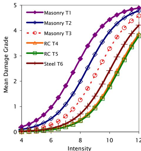
**Figure 7: Mean vulnerability curves for the principal typologies in the pilot region**
