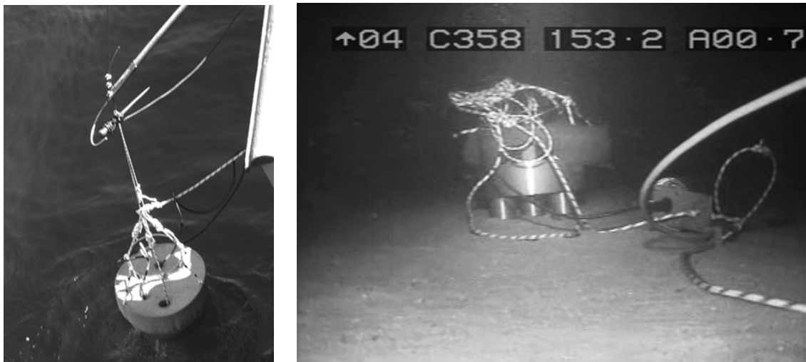
Figure 2. Left: OBS' immersion. Right: Submarine robot image from the OBS and the pressure sensor deposited on the seabed.
