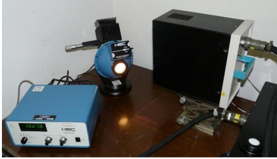
**Figure 4** Integrating sphere at ICGC calibrated by NPL.
