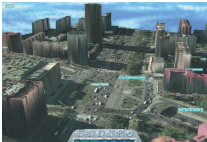
True orthoimages in combination with 3D visualization systems make it possible to navigate intuitively and interactively through the city.
