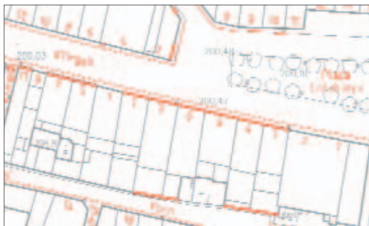
The photogrammetric stereoplotting data is shown in grey and the data incorporated from field revision in red.
