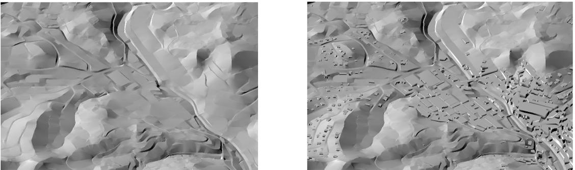
Left image shows hill shading using the Digital Terrain Model, right image shows the same area using Digital Elevation Model.
