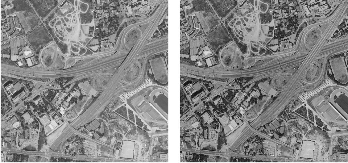
Left image shows an orthophoto rectified using a Digital Terrain Model, right image shows the same orthophoto rectified using Digital Elevation Model.
