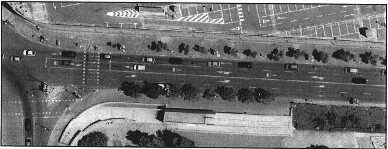
Figure 7. The top image shows a detail of an orthophoto rectified using a DSM obtained from LIDAR data. The bottom image shows the result using a DSM obtained by stereoplottting
