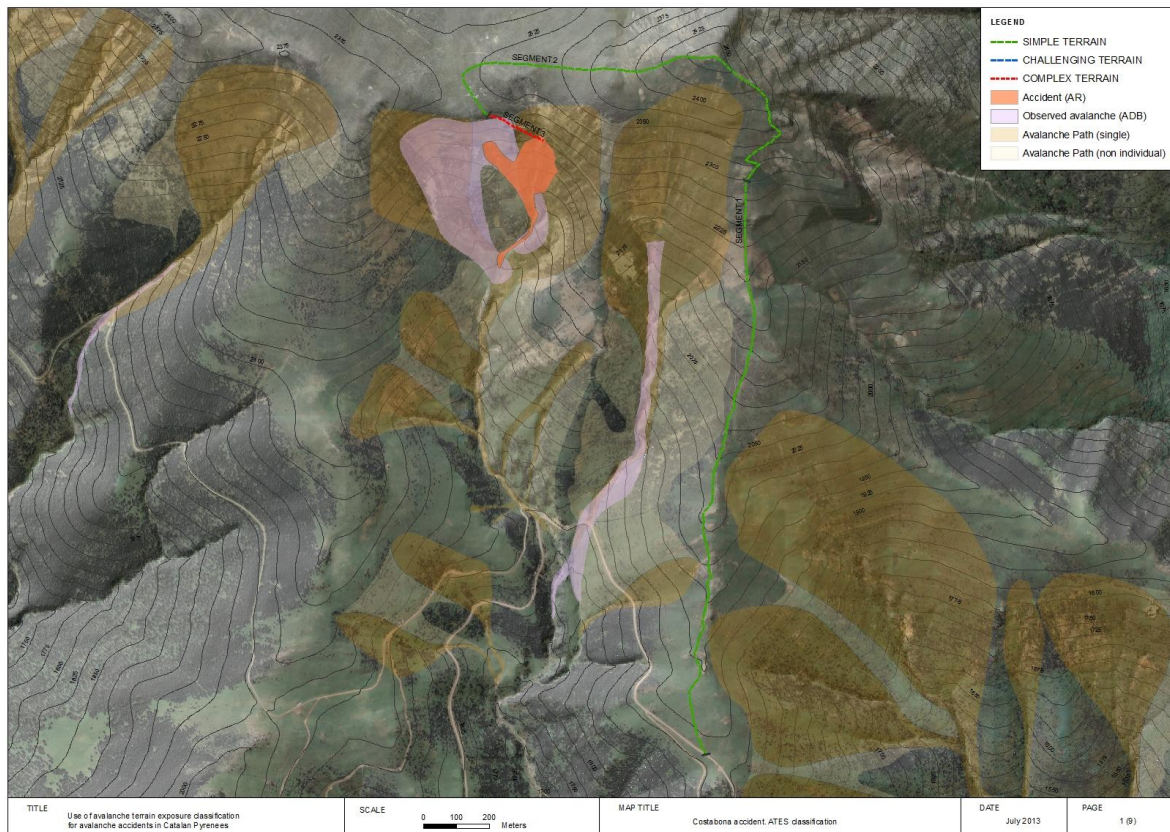
Figure 3: Map of Costabona accident with avalanche terrain classification: the two first segments of the track were classified as simple and the last one as complex, being this last one the place of the accident. In red colour we mapped the avalanche of the accident. As a background layers there are orthophotomaps and observed avalanches (in light violet) and avalanche paths in light orange, from ADB.
