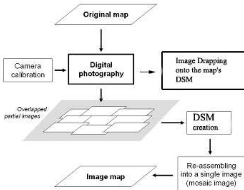
Fig.1. The flowchart of the transformation of the original map to its digital form and the necessary elaborations.
