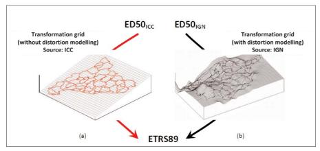
The distortion of the IGN transformation (shown with undulations) is due to the use of classical measuring methods. The ICC transformation does not distort the information because it was already constructed with GPS coherence at origin.
