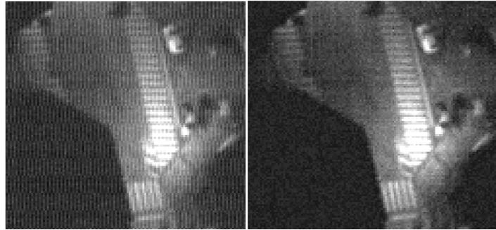
**Figure 9** Example of electronic noise pattern of panchromatic imaging (left) and the result after the spectral filtering.
