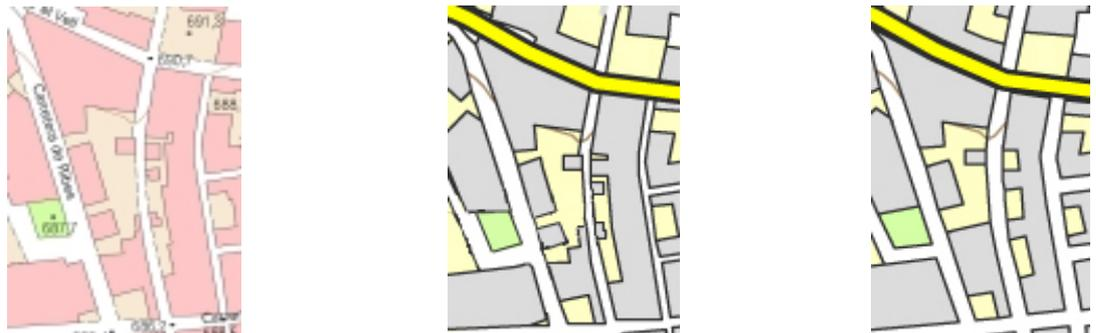
Figure 6.- Left figure shows the streets in the original data. Central figure shows the results after the automatic generalization and right figure shows the results after exaggerating the street width.
