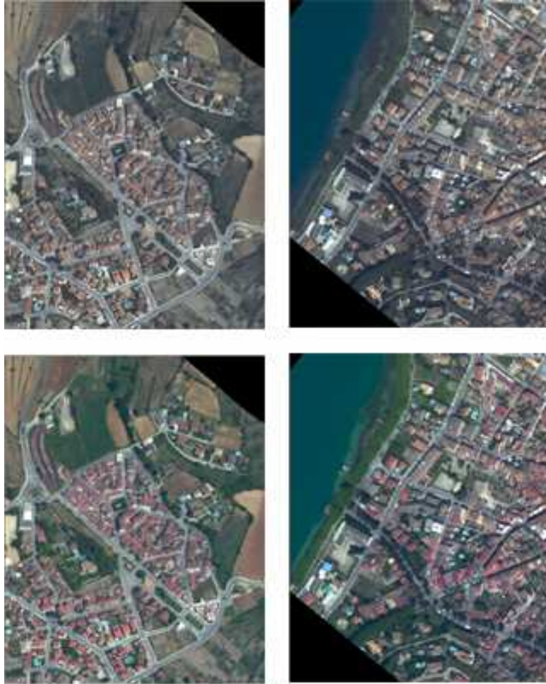
Figure 8. DMC colorimetric calibration example on Banyoles area from [30]. (Up) DMC images after absolute calibration derived from simultaneous CASI images. (Down) DMC images after colorimetric calibration.
