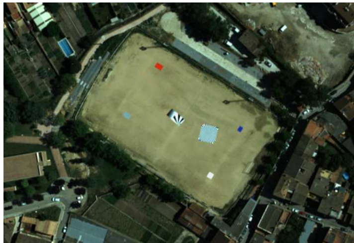
Figure2. ICC Banyoles (Spain) ICC test field with man-made covers and Siemens stars deployed (15 July 2008).
