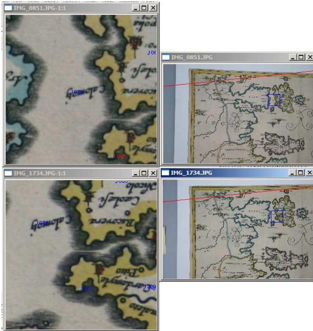
Fig. 5. Matching process. The red labeled point has been extracted from the DSM generation as a bad match according to the epipolar geometry constrain.
