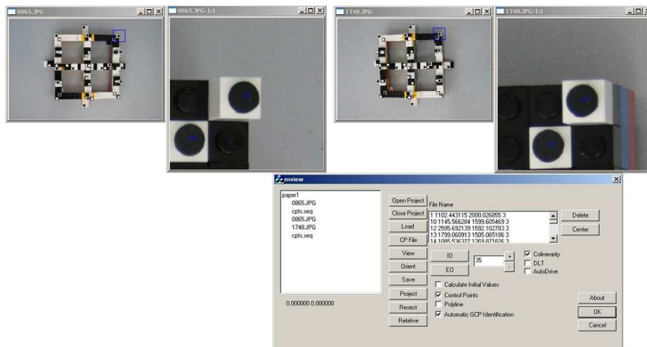
Fig. 3. Control points' field image collected for the determination of the calibration and the exterior orientation parameters
