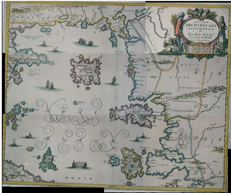
Fig.6. Final orthomosaic. No bending has been applied, on purpose, in order to distinguish the separate tiles of partial orthoimages.
