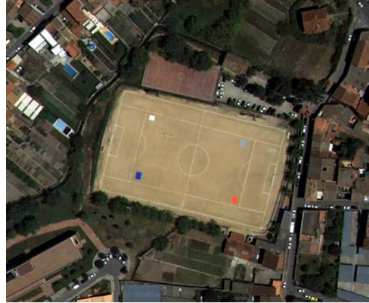
Figure 2 Aerial photo of the targets specifically deployed for radiometric validation.
