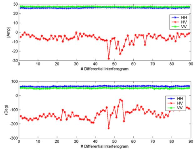
**Fig13:** Amplitude and Phase temporal evolution of a Trihedral placed at 600m from the sensor from 5pm on Dec.18<sup>th</sup> to 9am on Dec.19<sup>th</sup>.
