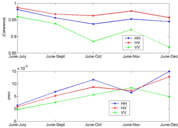
**Fig11:** Urban Pixel Coherence and vertical displacement profile in the Coherence-Based Approach.
