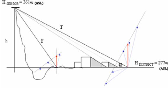
Fig.3: GBSAR acquisition geometry.
