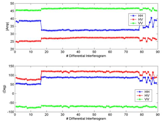
**Fig12:** Amplitude and Phase temporal evolution of a high reflectivity urban pixel from 5pm on Dec.18<sup>th</sup> to 9am on Dec.19<sup>th</sup>.
