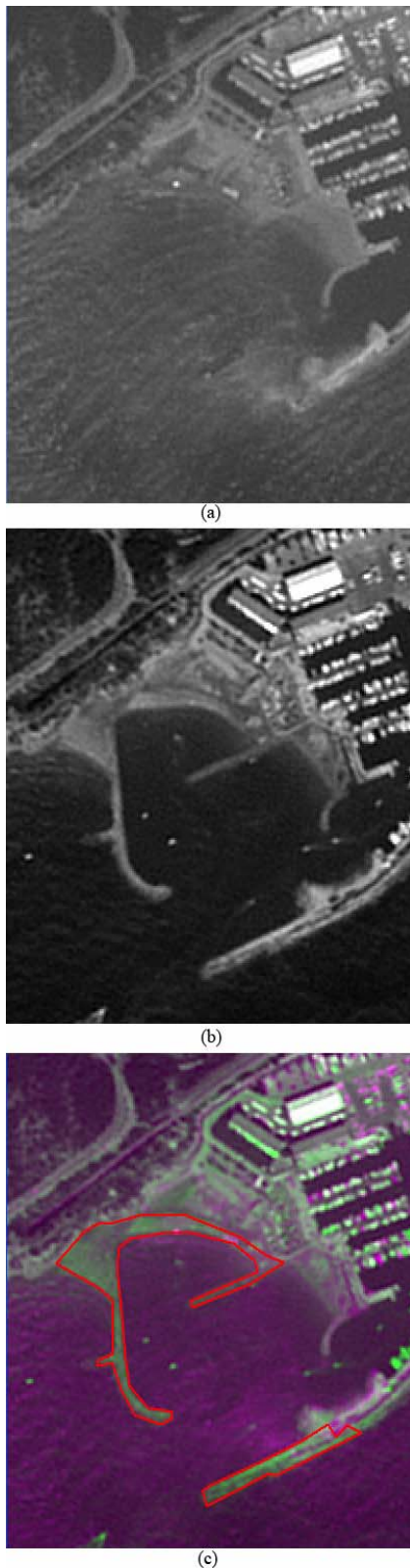
Figure 3. Example of a change on Garraf area from water layer to harbor. (a) 17-05-2006 pan SPOT image. (b) 03-09-2006 pan SPOT image. (c) Delineated change on a RGB multitemporal image.
